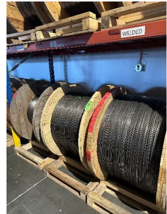
Welded Quarter Inch Capillary Tubing
